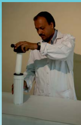
Candle used in Domestic Water Purifiers
